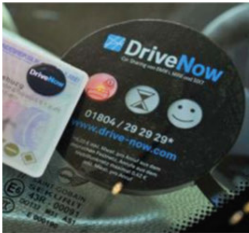
Outer reader with status display for Car Sharing
